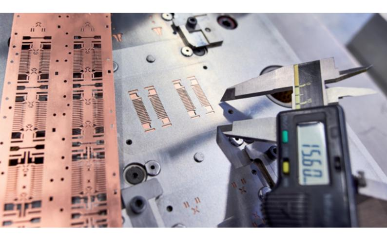
The combination of metal and plastics and the assembly of electronic components requires a variety of different technologies, such as stamping, etching, electroplating, injection molding, automated handling and verification processes.
